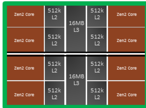
Figure 2 Two Core Complexes (CCXs) on a Core Complex Die (CCD)
